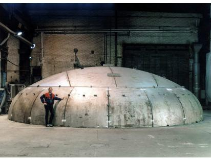
Deform has made a large number of pressure vessel heads to pulp digesters worldwide. The biggest so far is a head of  $\emptyset$ 13200x46,5 mm (1.4462). It was made of 20 petals and 8 crown parts. Above impressive fit at the pre-assembly!
